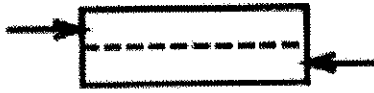
Figure 3. In loading to determine shear capacity of timber the forces are applied at each end.
