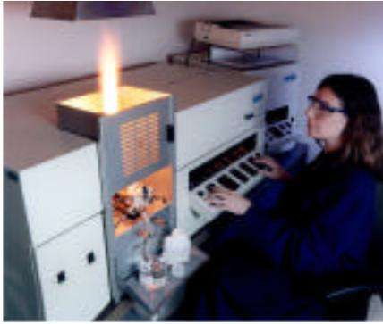
Fig. 3. The atomic-absorption spectrophotometer is often used to perform quantitative elemental analysis. A solid is placed in solution and is then aspirated into a heat source, so that it can be measured. Elements can be identified by their signature wavelength, and the absorption of light by the aspirated atoms can be measured and quantified.
