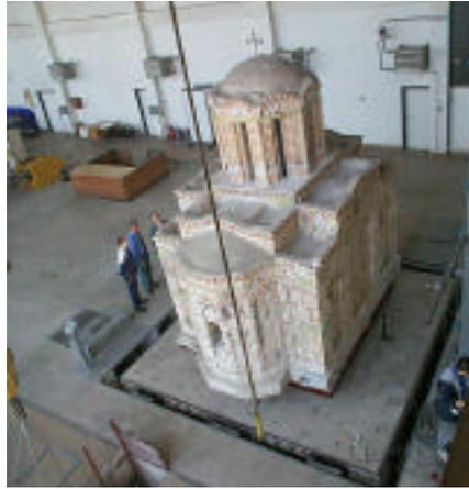
Fig. 4. Testing of a 1:2.75 scale model of the Church of Sveti Nikita near Skopje, Macedonia, at the Institute of Earthquake Engineering and Engineering Seismology in Skopje (IZIIS). For a detailed discussion of this testing refer to Kelley, Gavrilović, and Šendova. "A Study of Seismic Protection Techniques for the Byzantine Churches of Macedonia," *APT Bulletin* 34, no. 2-3 (2003): 63-69.
